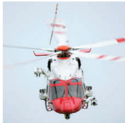
The SAFIRE 380-HD EO/IR sensor pod is mounted to an Augusta Westland AW189 helicopter.
