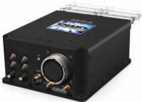
The General Micro Systems SB1102-HDVR Eagle is a small-form-factor rugged video recorder and workstation processor able to capture four independent HD-SDI 1080p video channels at 60 frames per second.
