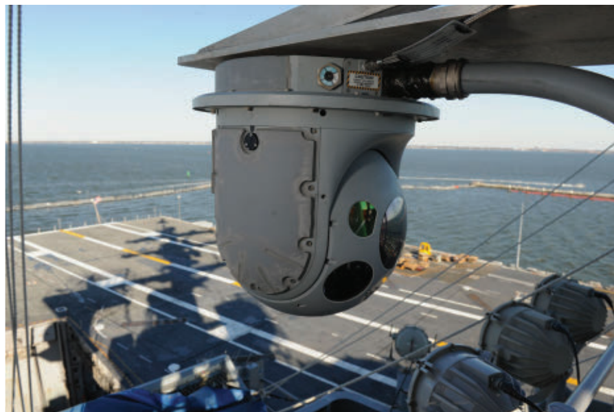
The Navy's experimental Situational Awareness System (SAWS) uses two EO/IR sensors placed forward and aft of an aircraft carrier's island to provide 360-degree surveillance capability.
